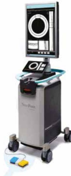
NvisionVLE® Imaging System. Advanced OCT for evaluation of human tissue microstructure.
